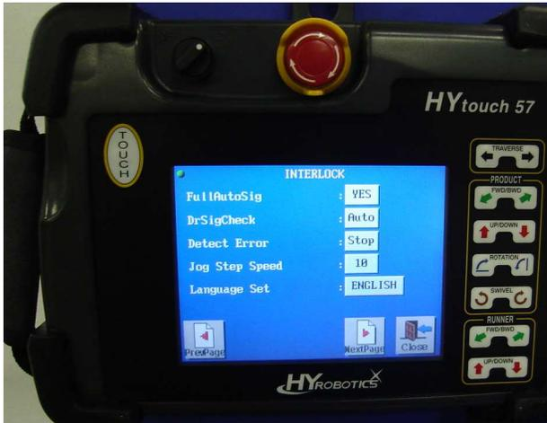
**Do not change this setting unless if required by Manufacture, Each model is has different value**
