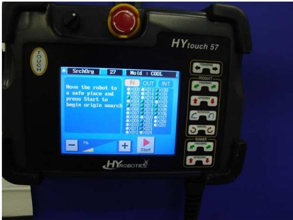
After read all TP, NAND, TP and turn on Servo Motor and check each sensor Robot will goes to servo motor origin point.
