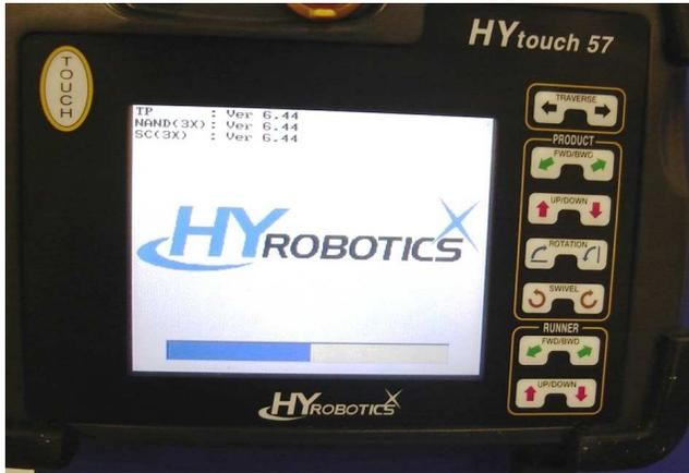
As long as robot read all 3 program version , and blue bar goes all the way goes to end of white bar means robot Handy Controller, Main controller and communication is working properly between.
