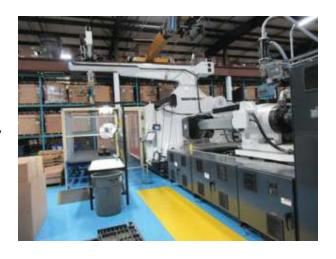
The 1,300-ton Maxima, coupled with a Cartesian robot from HyRobotics, is currently molding the front panel for a pump housing for the energy/fuel market. Carinci said the machine will probably be the largest the facility acquires. Before the plant brought it online, Statesville's largest press had 1,100 tons of clamping force.
