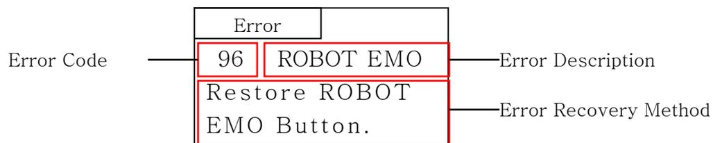
Error cause Alarm and Buzzer, display the error message
