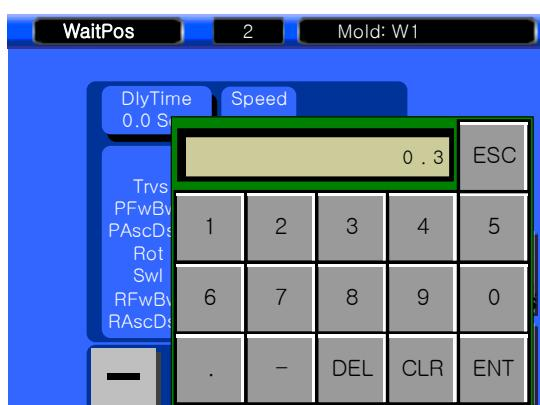
Make input by pressing **0**, **.**, **3** in regular order, store delay time by pressing **ENT**, and then close window.
