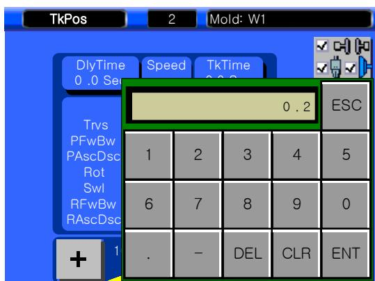
Make input by pressing **0**, **.**, **2** in regular order, store delay time by pressing **ENT**, and then close window.
